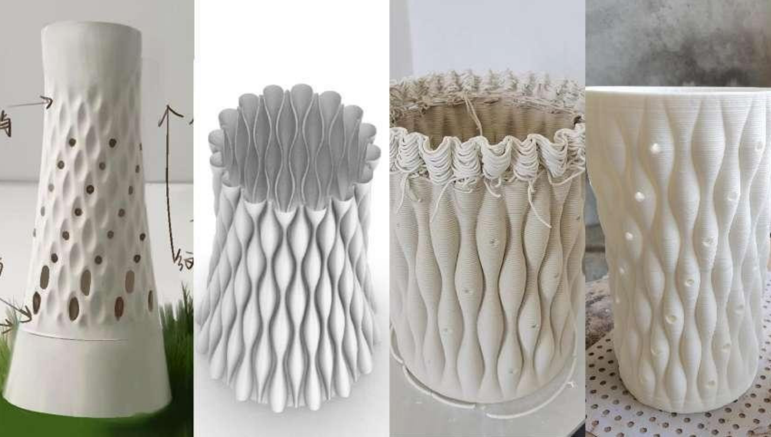
Figure 17. Development of Honeycomb Lamp Forms and 3D Printing Optimization Process (Designed and Photographed by the Author).
